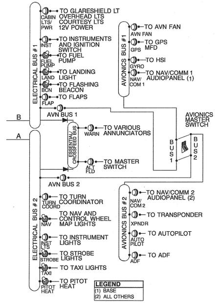
Figure 7-7A. Electrical Schematic (Serials 17280984 and On) (Sheet 1 of 2)
