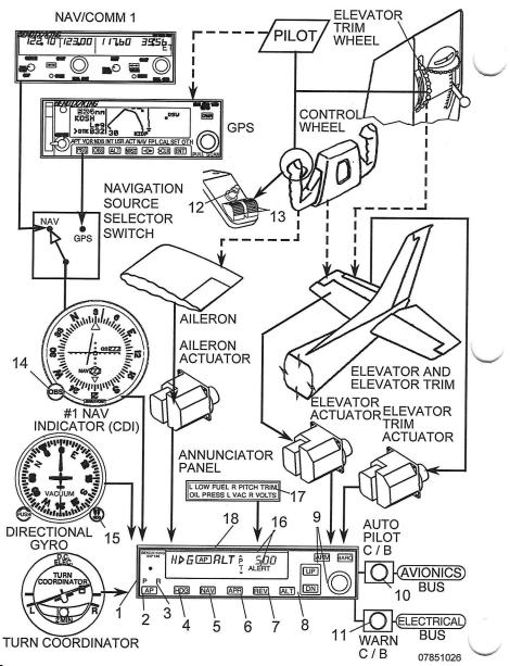
Figure 1. Bendix/King KAP 140 2 Axis Autopilot Schematic (Serials 17280831 thru 17281173) (Sheet 1 of 2)
