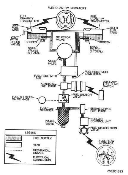
Figure 7-6. Fuel System Schematic (Sheet 1 of 2) 17280001 thru 17281187
