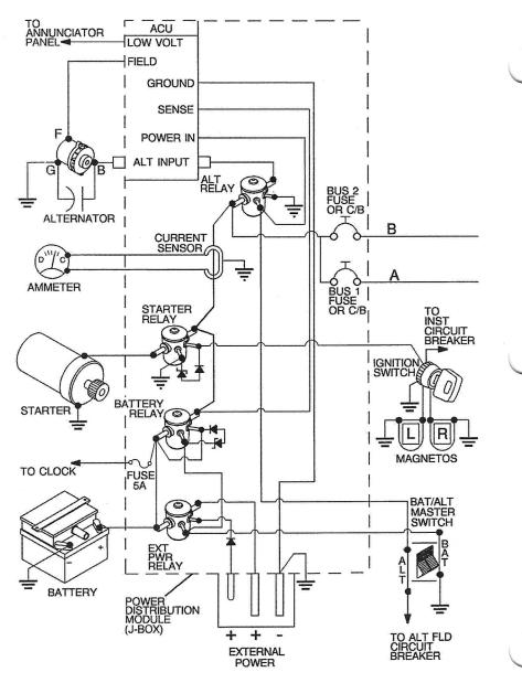
Figure 7-7A. Electrical Schematic (Serials 17280984 and On)(Sheet 1 of 2)
